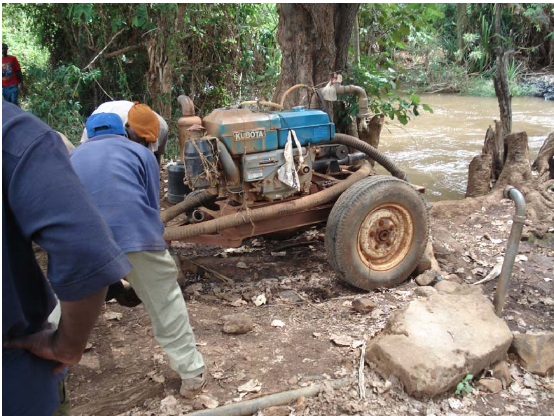
Plate 10: Water abstraction along Rupingazi River using a portable pump
